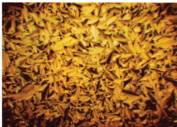
Figure 7. Photomicrograph of the SmA phase, with a focal-conic texture, of compound 3a at 141.3°C in the cooling cycle.
